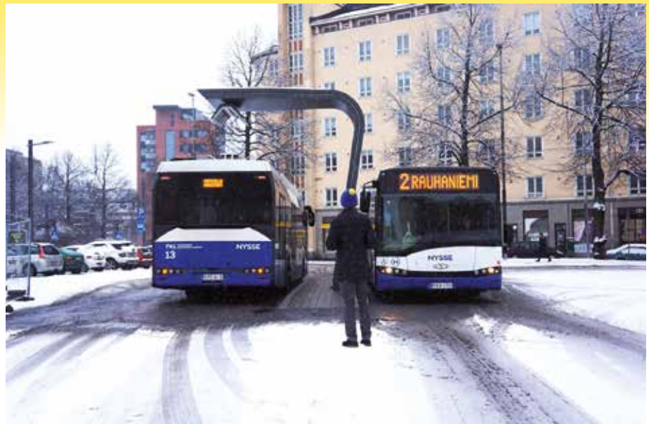
Figure 2: In Tampere, measuring devices have been installed in four electric buses and one hybrid bus to help monitor electricity consumption. The data will be used, for example, for route planning and the electrification of public transport. The charging station is located near the city center in Pynnikipintori square. Due to winter conditions, there is heating under the asphalt of the charging station. Credits: Anna Vilhula e Angelique Lusuan.
