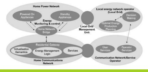
an operator network. The residential gateway selects and conduits information to the proper device interface, applies the necessary centralized control logic, and enforces rigorous communication encryption.
